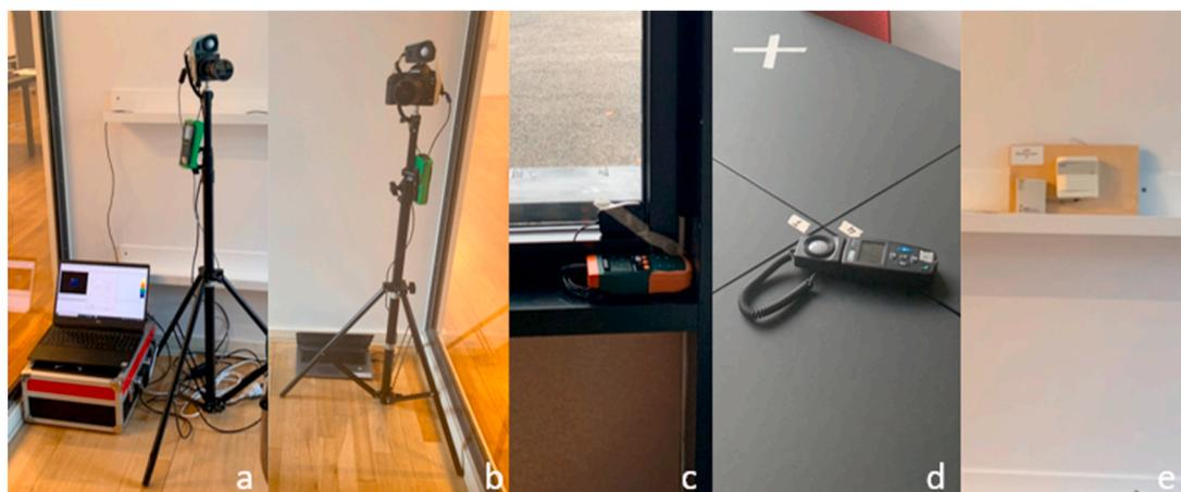
**Fig. 7.** Photos of the equipment. a) LMK image-resolved photometer equipped with lux meter for control, b) home-calibrated Canon image-resolved photometer equipped with luxmeter, c) vertical illuminance lux meter at the window, d) horizontal luminance lux meter at the table, and e) HOBO together with VAISALA indoor measurement station.
