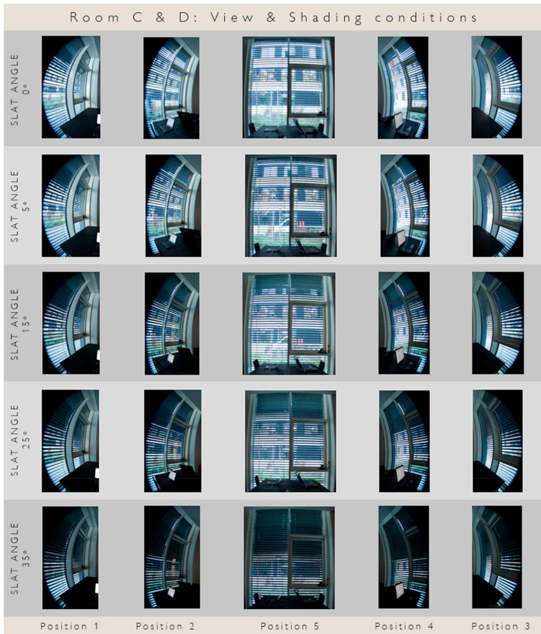
Fig. 5. Cropped Fisheye images from each position showing the each window view condition through different solar shading in room C. The shading conditions were identical in room D but the view was different.
