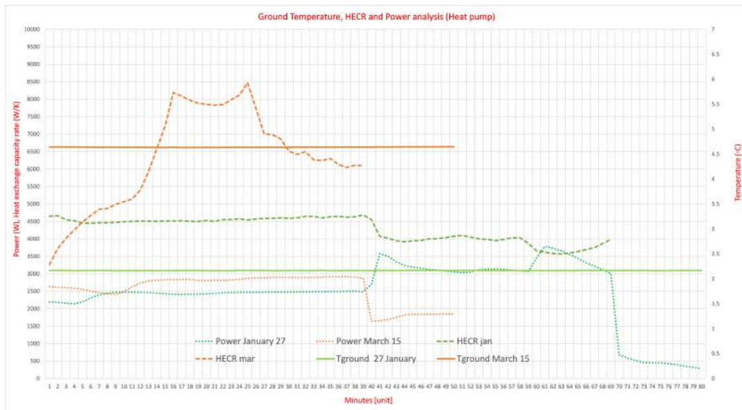
Figure 2.27: Analysis Tground, Power and HECR, HP in operation.
