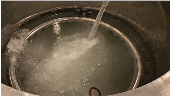
Figure 4. Ice slurry generated by the ISHP.
