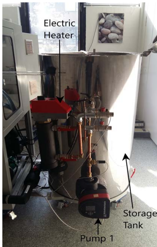
(a) Loop simulating the solar collector
