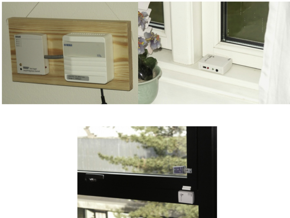
Fig. 2. Pictures of the instruments used to measure the indoor environmental variables and window opening behaviour. Top left: CO 2 monitor connected to a data-logger with built in temperature, relative humidity and illumination sensors. Top right: Window state sensor (open/closed). Bottom: window state sensor (open/closed) and window position sensor.
