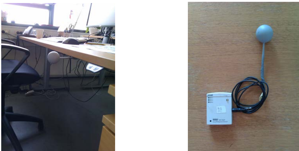
Figure 1. (Left) Placement of the operative temperature sensor at workplace, (Right) A set of grey sphere-shaped sensor and data logger
