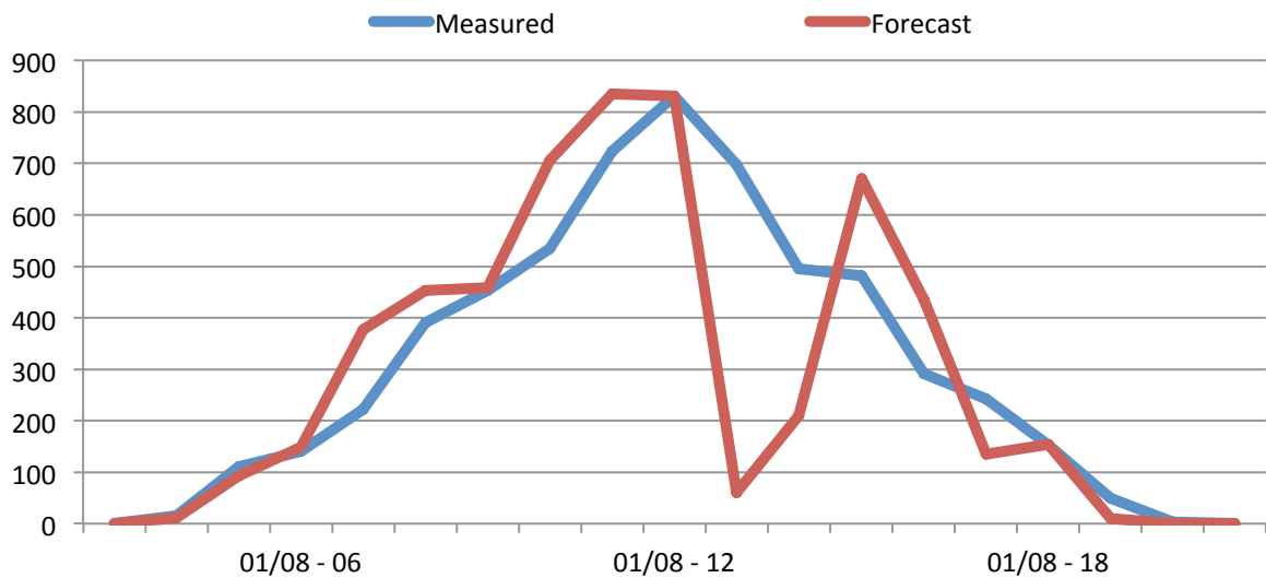
Figure 7-10 - Largest solar radiation underestimation
