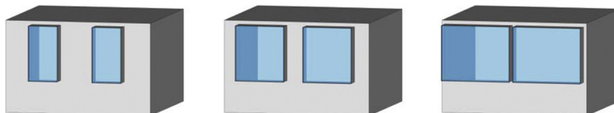
Fig. 1. Illustration of glazing-to-floor-ratio for a 4 m × 4 m room. From left to right: Glazing-to-floor ratio of 15%, 25% and 35%.
