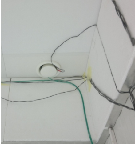
Figure 3.7: Exhaust diffuser used for the experiments.
