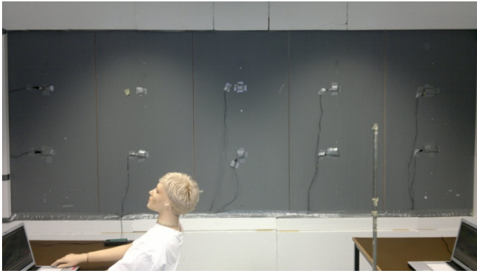
Figure 3.1: The simulated window with the sensors attached for surface temperature measurements.
