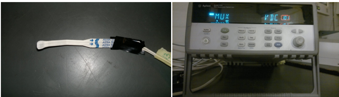
Figure 3.20: Craftemp Astra thermistor (left) and data acquisition unit Agilent (right).
