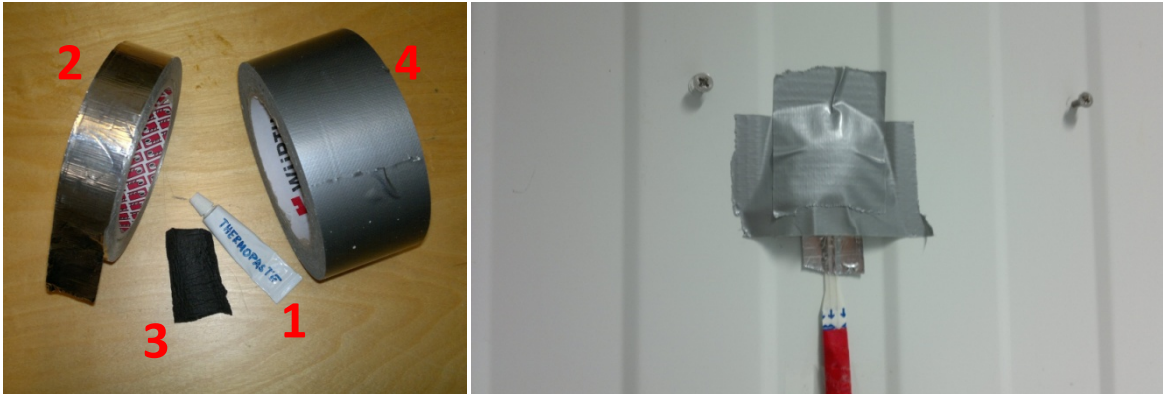
Figure 3.25: Components used to improve the conductivity and accuracy of the surface measurements (1 – thermal paste, 2 - silver tape, 3 – insulation strip, 4 – duct tape).
