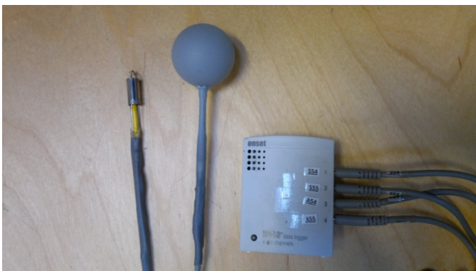
Figure 3.19: Sensors for the operative temperature (sphere) and air temperature measurements and HOBO data logger.
