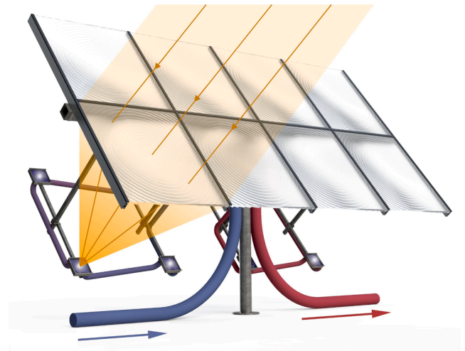
Fig. 3. Illustration of the Heliac concentrating solar collector. Fresnel grooves are enhanced for visualization.
