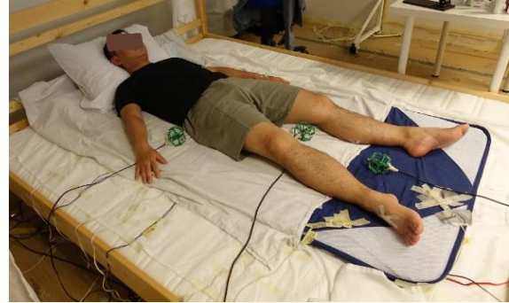
Fig. 1 - View of a subject lying on the VM and the three temperature sensors positioned around the subject (placed inside green protectors). The white surfaces near the feet are where the suction openings of the VM were.
